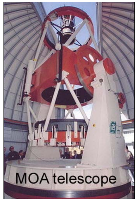
The 1.8m MOA telescope at The University of Canterbury's Mt John Observatory is the largest optical telescope in New Zealand and the largest in the world dedicated to searching for microlensing events.
