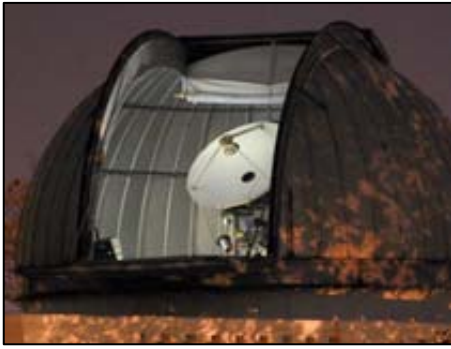
This modest rooftop radio dish, only 4 feet (1.2 m) across, has mapped the presence of carbon monoxide in giant clouds throughout the galaxy.
